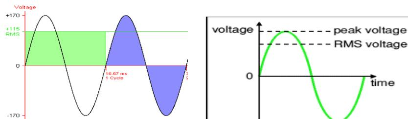
For a pure sine wave the equivalent RMS value is 0.707 times the peak value. Conversely the peak voltage can be calculated as 1.414 times the RMS Value.
