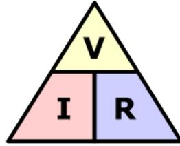
For example: if you have a 12-volt battery connected across a 6-ohm resistor the current flowing would be 2 amperes.
