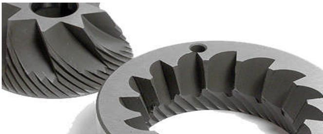
Burr grinders are nearly identical to stone grinders except their grinding wheels are made out of steel with small burrs protruding out the sides (sometimes called "teeth") which shear the grain into flour. Burr grinders have some advantages and disadvantages over stone grinders.
