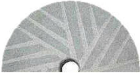
Stone Grinders are the oldest type of grinder there is. Stone grinders have two circular grinding stones. One stone turns against a stationary stone. When grain is ground, it falls through a channel into the center of the two stones. As the stone rotates, it pulls the grain out through the channels where it is ground. The flour falls out the outer edges of the two stones.
