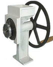
**The Country Living Grain Mill** is made in the USA and built like the proverbial "tank." Quality is outstanding, from its stout cast metal housing and sealed ball bearings to its huge 5" precision steel burr plates and robust handle and fly-wheel. Turning effort is very easy
