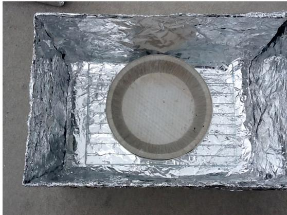
4. Make a rack to hold your cooking rack. I used 4 pop cans to try it out. Since I know the oven works, I will use some coat hangers or other wire pushed through the box to hold up my cooking rack.
