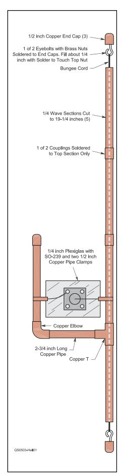
Figure 1—The assembly drawing for the VHF/UHF folding J-pole antenna.
