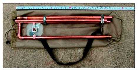
Figure 7—The completed folding J-pole, ready for packing.
