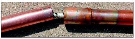
Figure 4—The bungee cord runs through each of the antenna elements.
