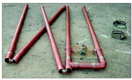
Figure 6—The J-pole in the process of being "folded."
