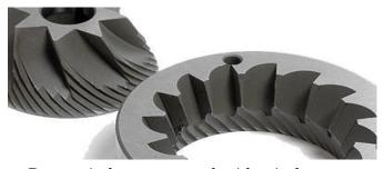
Burr grinders are nearly identical to stone grinders except their grinding wheels are made out of steel with small burrs protruding out the sides (sometimes called "teeth") which shear the grain into flour. Burr grinders have some advantages and disadvantages over stone grinders.
