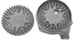
Impact grinders use rows of 'blades' placed in circular rows on metal wheels. One wheel turns and the other wheel is stationary, like the stone grinder. The rotating wheel turns at several thousand RPM. As grain is fed into the center of the fixed wheel, the interaction between the two wheels 'impacts' the grain and pulverizes it into fine flour as the grain works its way to the outside of the wheels.
