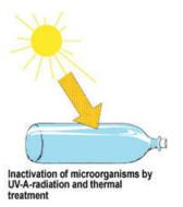
Solar water disinfection is a simple method to improve the quality of drinking water by using sunlight to inactivate pathogens causing diarrhea.
